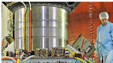
Cordell Grant integrates two BRITE satellites with the PSLV-C20 launch vehicle in India on Feb. 15, 2013. The satellites, enclosed in their XPOD separation systems with protective panels still on, can be seen angled upward on either side of the upper stage of the rocket. (Indian Space Research
