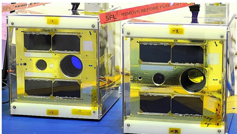
The BRITE satellites designed at the Space Flight Laboratory of the University of Toronto Institute for Aerospace Studies will orbit Earth every 100 minutes or so and measure the brightness of stars to learn more about their volatile inner workings. (Courtesy Cordell Grant)
